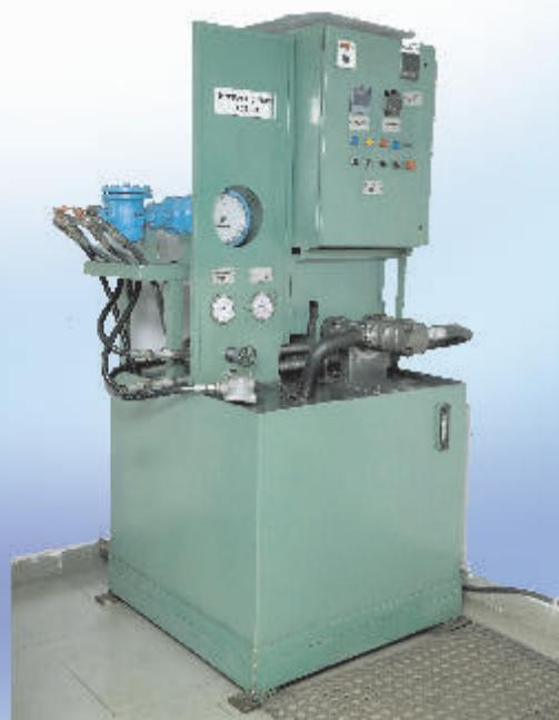
Hydraulic Pump Testing Machine
